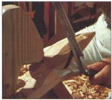
After body is roughed out with a bandsaw, the general shape is formed with a draw-knife and spokeshave.
